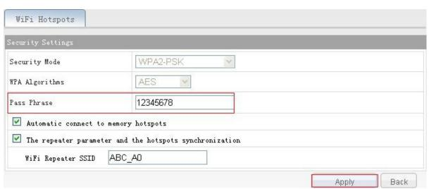
Input the correct password, confirm it is correct one, then click Apply button.
