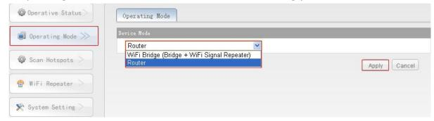
Choose Router Mode can switch LAN, WAN port to fit for different environments connected to Modem, the default is the ethernet cable is LAN port, RJ45 ethernet port is LAN port, see the following pictures:
