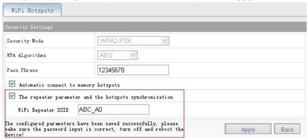
Click Apply button, the above interface will appear, the configured parameters have been saved successfully, please make sure the password input is correct, turn off and reboot the device.
